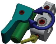
On the underside of the base plate there is another screw. Through this you can adjust the tilt of the trigger plate.
