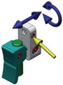
By the top screw, the trigger is attached to the trigger bar of each match gun. The trigger is continuously movable in longitudinal direction of the weapon and can also be swung sideways. By tightening the screw the trigger can be locked in its desired position.
