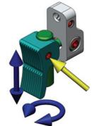
The trigger plate can be infinitely adjusted in height and can be rotated around the vertical axis by releasing the side screw.
